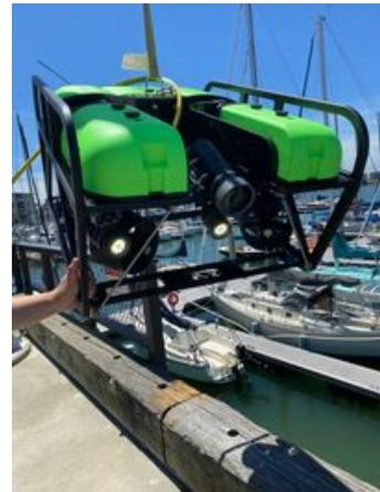
Before the in-water testing, we do a pre-dive check of the vehicle to make sure that everything is functional. Some important parts that we focus on are the: thrusters, flotation, cables/whips, and sealing surfaces. After everything looks good during the pre-check, launch and start the wet/operational test.
