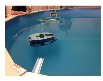
P150s which are used in outage support and tank inspections.
